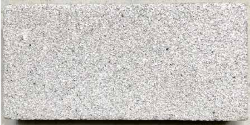
Sample K6-17 after sandpapering test
